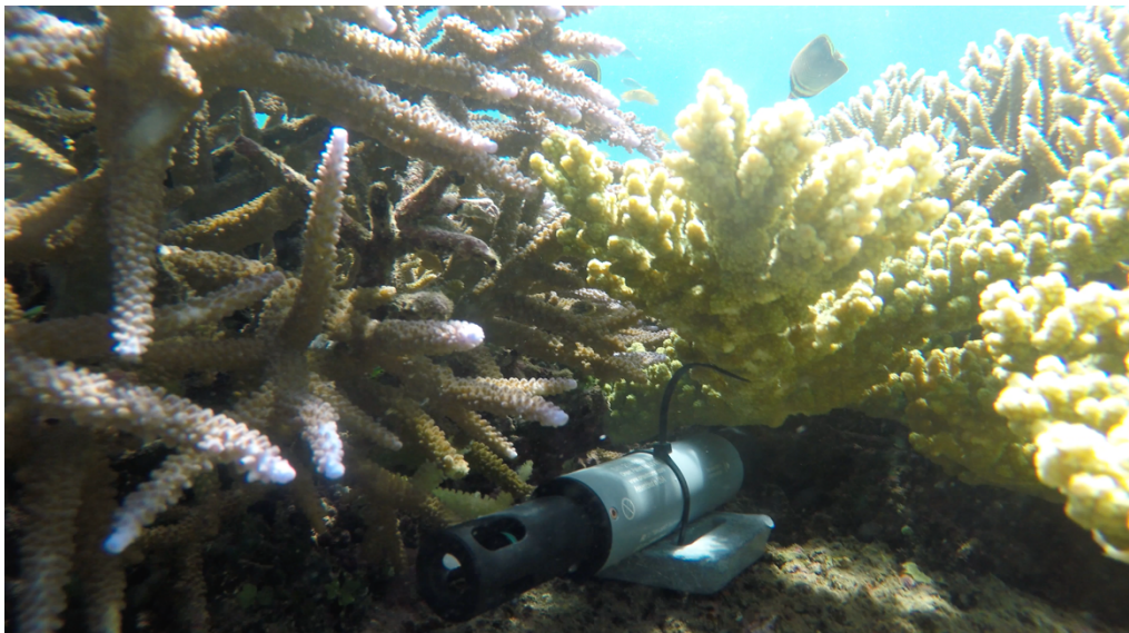
Figure 4. The HOBO U26-001 oxygen logger deployed adjacent to branching corals of genus Acropora .
